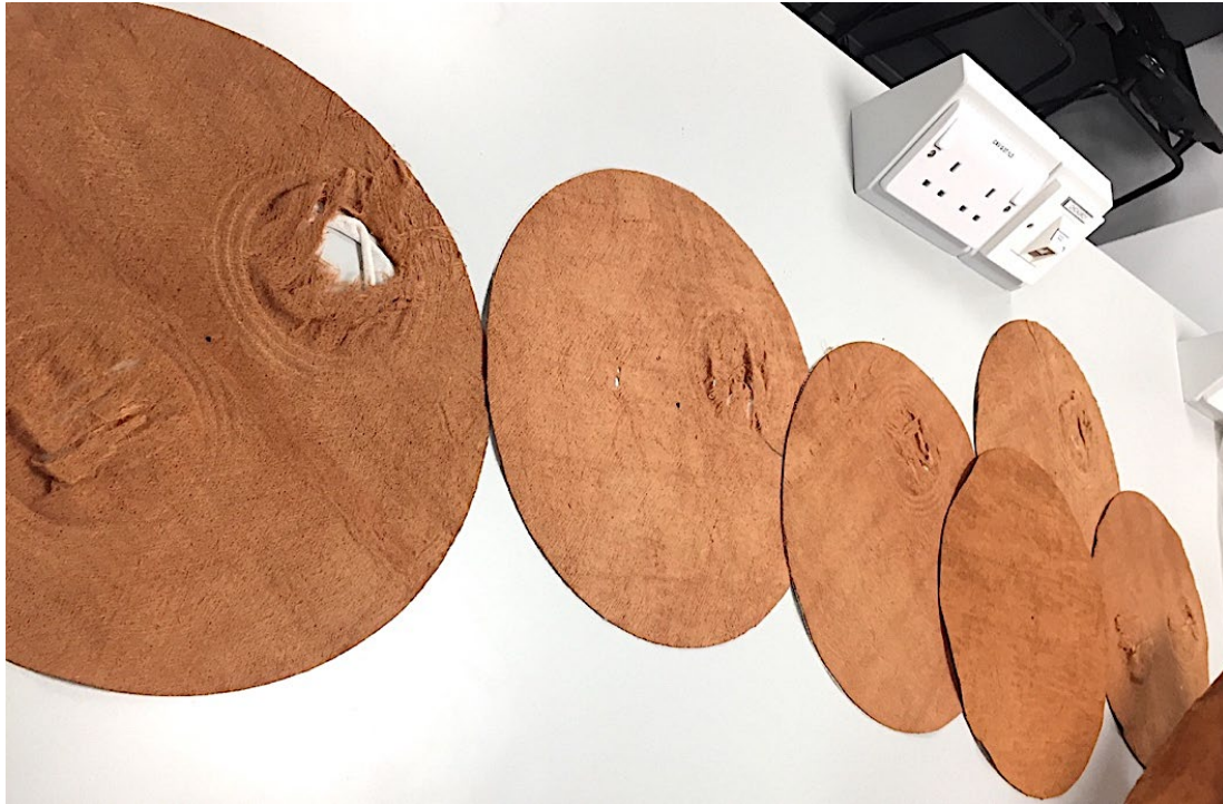
Fig 9. Burst tests at MMU textiles laboratory, to measure barkcloth's strength.
